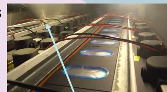
Liquid Electrolyte Spewing at time of Cell Venting
