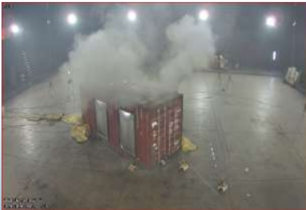
TR propagation for 3 hours [TR + 00:11:54]
