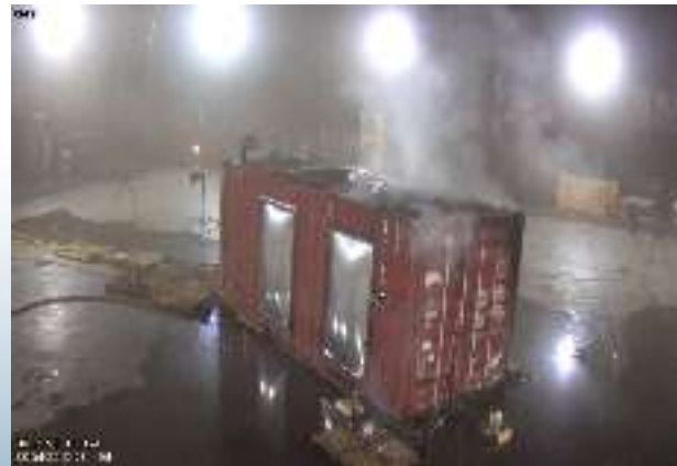
TR propagation continues after water flow restart [TR + 01:49:54]
