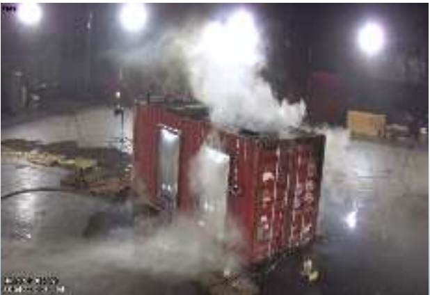
TR propagation after water flow off [TR + 01:13:05]
