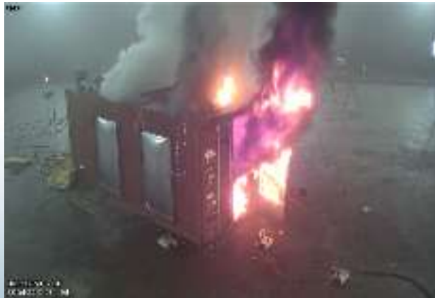
Flashover conditions and flaming from open door [TR + 02:09:48]
