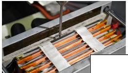
Adding thermal mass of the copper plates mitigates cascading failure.
