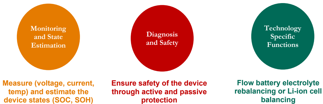
Figure 3. Device Management System Functions
