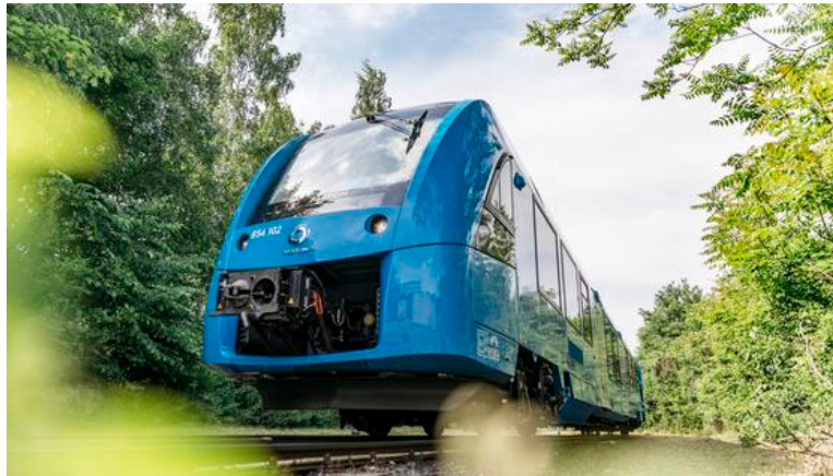
Figure 12: Coradia iLint hydrogen powered train Saxony Germany [30]
