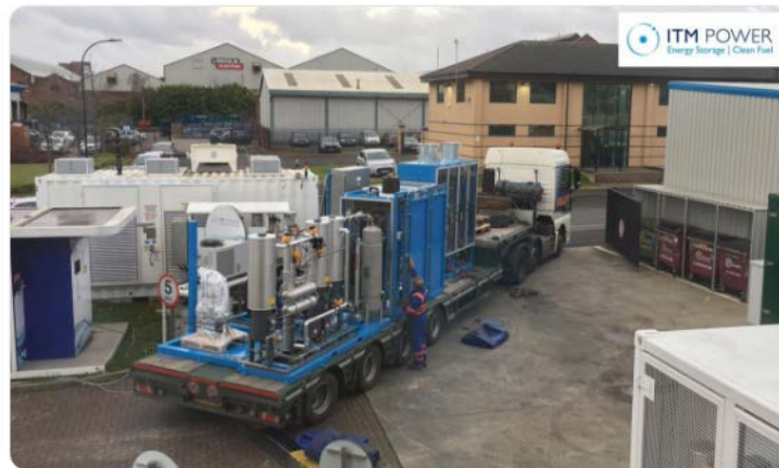
Figure 4. ITM Power 1 MW electrolyzer
