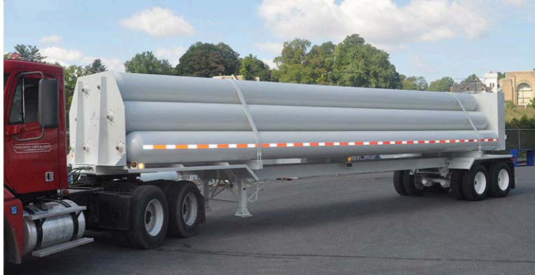
Figure 5. Photo of hydrogen gas cylinders on a tube trailer [15]
