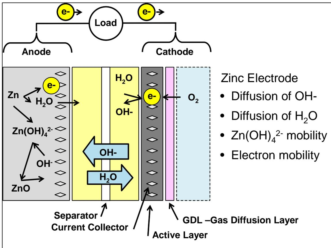
Figure 64. Zinc-air Battery Functional Schematic
