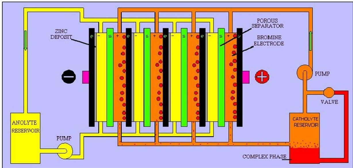
**Figure 56. Zinc-bromine Cell Configuration**
