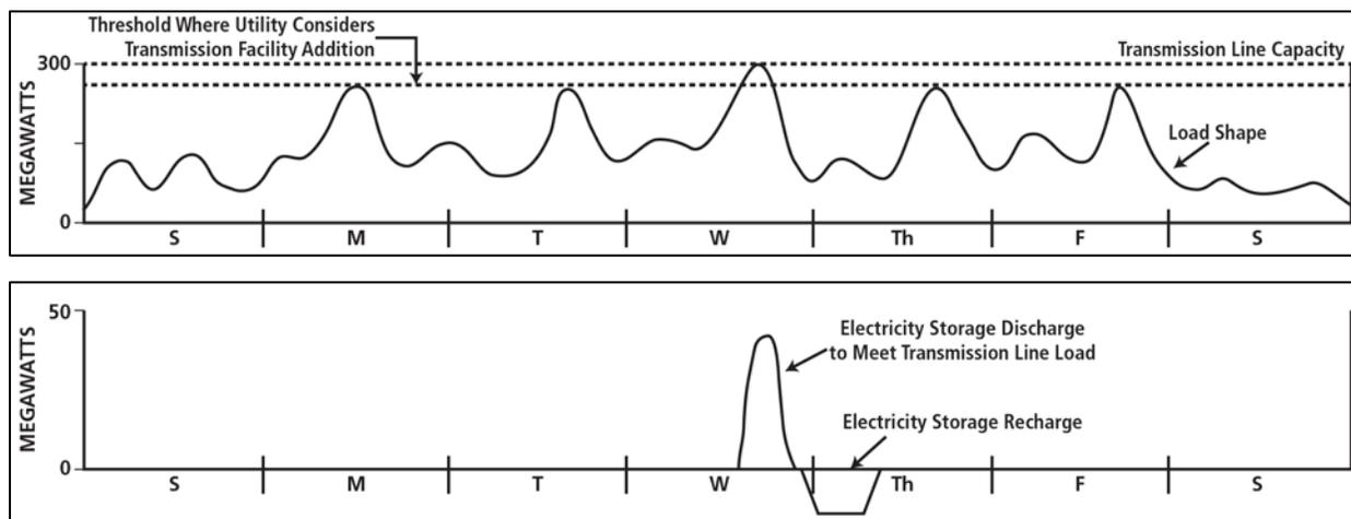
**Figure 11. Storage for Transmission and Distribution Deferral**
