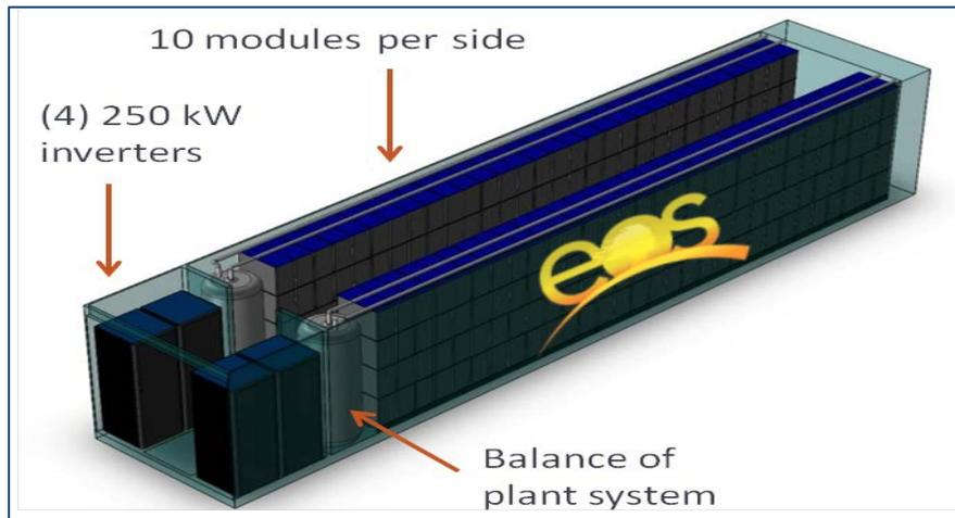
**Figure 66. Illustration of 1-MW/6-MWh Eos Aurora Zinc-air Design**
