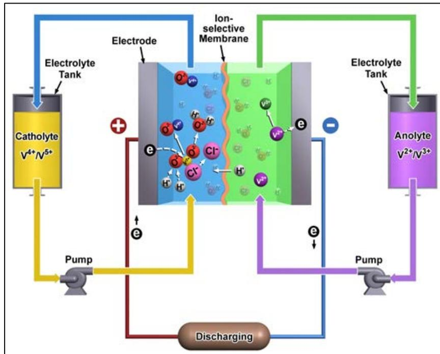
**Figure 45. Principles of the Vanadium Redox Battery**
