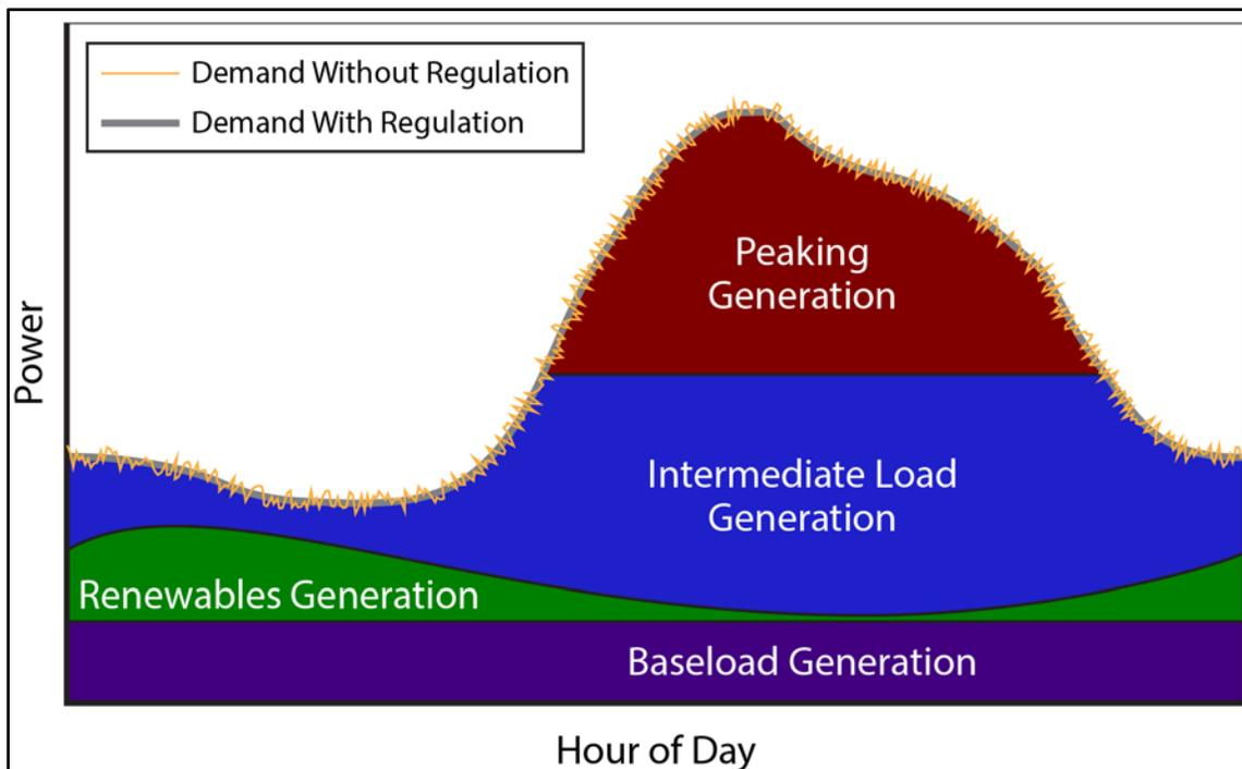
**Figure 3. System Load Without and With Regulation**
