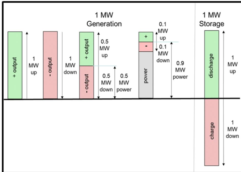
**Figure 4. Storage and Generation Operation for Regulation**
