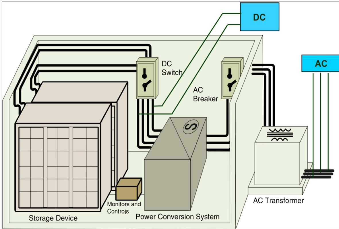
**Figure 1. Schematic of a Battery Energy Storage System**
