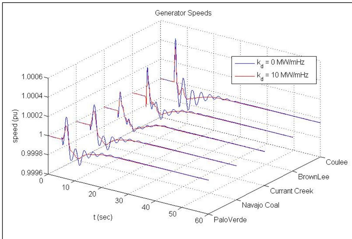
**Figure A-11: Generator Speeds at Five Buses in the WECC With/Without Damping Control**
