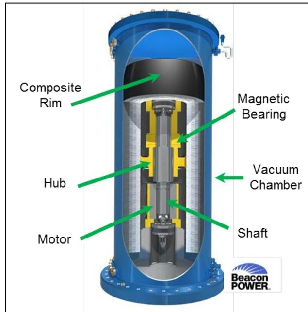
**Figure 89. Integrated Flywheel System Package Cutaway Diagram**
