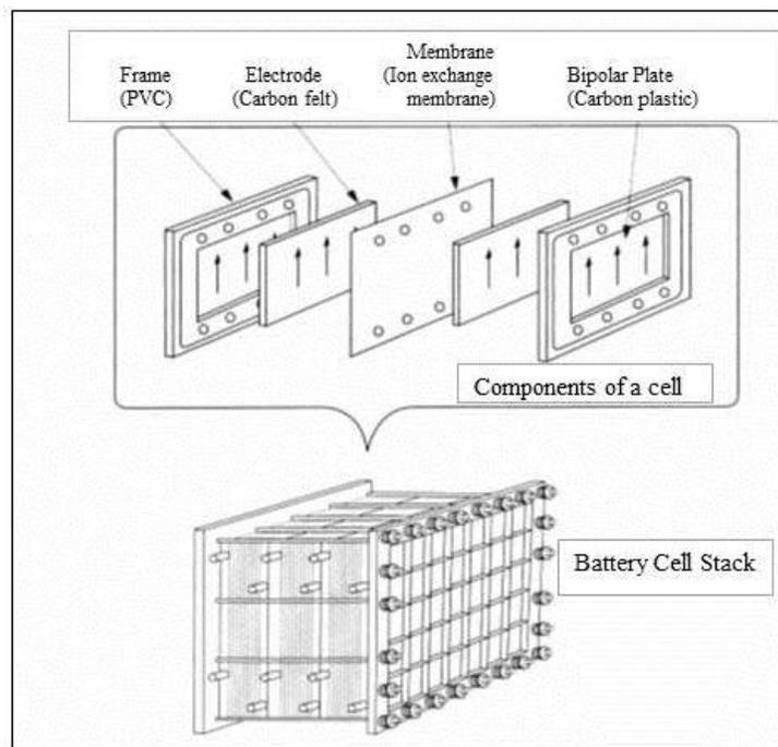
**Figure 44. Construction of a Vanadium Redox Cell Stack**
