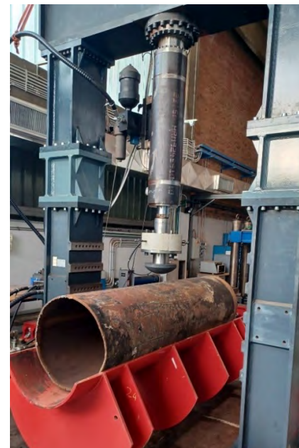
TEST SETUP FOR MAKING DENTS IN 26" VINTAGE LSAW
