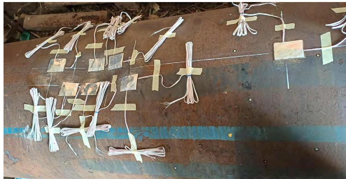
SG instrumentation on the damage area of one 24" specimen
