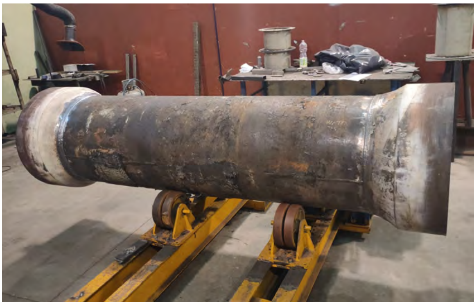
26" specimen with welded endcaps
