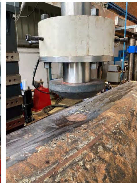
TEST SETUP FOR MAKING DENTS IN 26" VINTAGE LSAW
