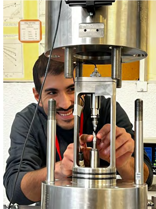
Vertical gas pressurized tensile test machine for sub- size specimens
