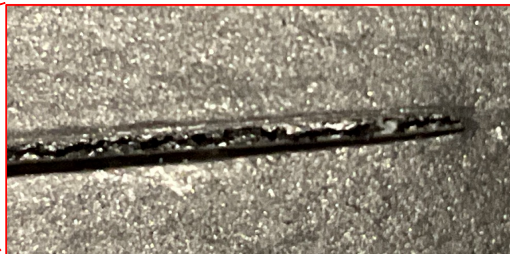
Notch 2 (weld seam), heat-tinted
