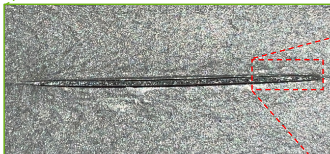
Weld Seam Notch
