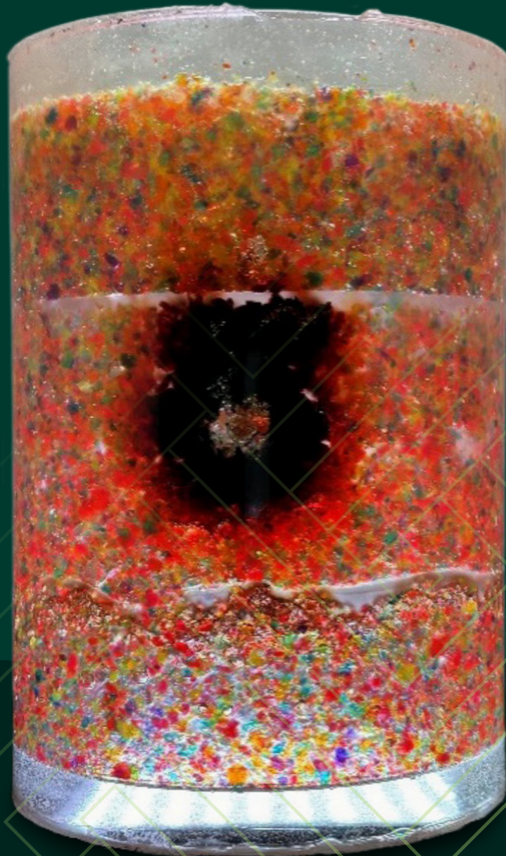
A container protected with Sandia’s “Bleeding Materials & Enclosures” product indicates a tamper attempt. In this image, silicone is used to encapsulate the air-sensitive beads.
