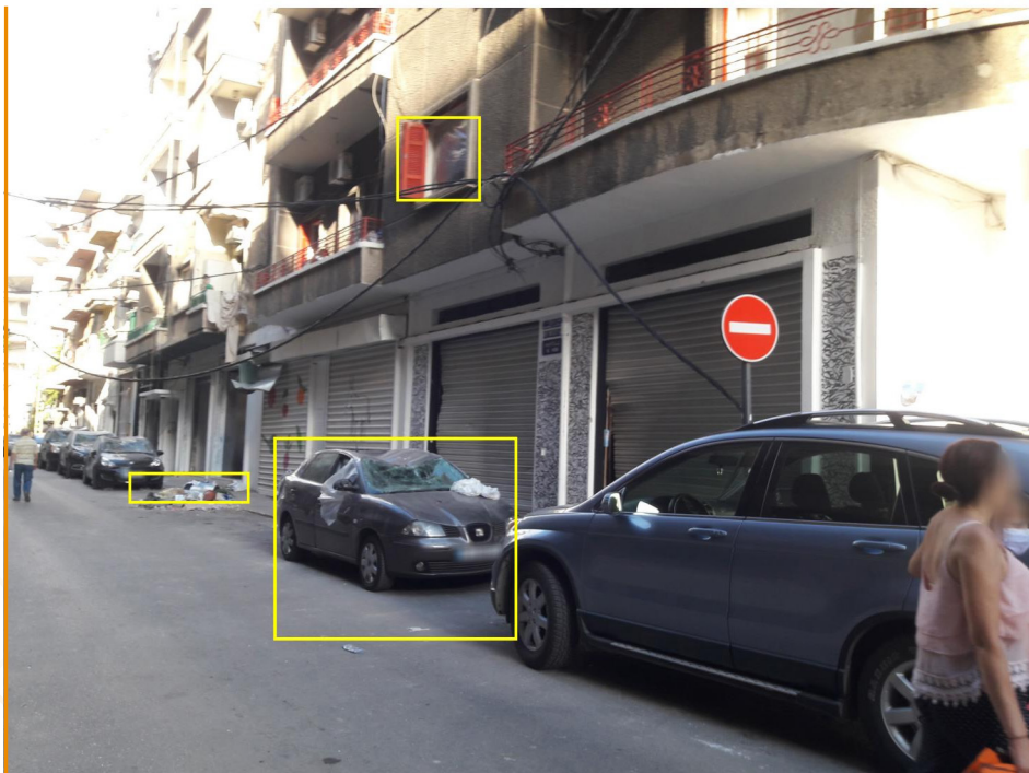
A VLM detecting and describing damage in Beirut. The damage was classified into eight categories and converted into blast over-pressure estimates for that location.
