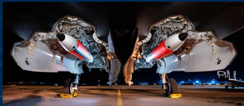
Two B61-12 joint test assemblies loaded on an F-35 aircraft for a flight test on Aug. 19, 2025. (Photo by Craig Fritz)
