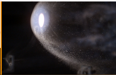
High-speed color image capturing a preheated thermal protection system sample during a hypersonic shock tunnel test.
