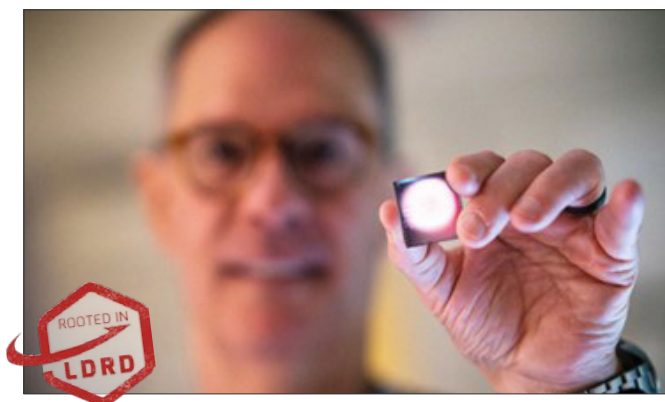
The Pre-Symptomatic VOC Detector of Seizure Events is a portable instrument that can alert the wearer to an imminent seizure more than 20 minutes before it occurs.
