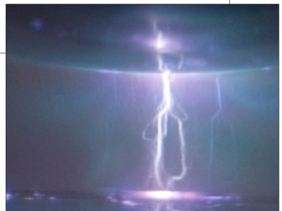
Full time exposure of electrical discharge between hemispherical anode (upper region), intervening insulator, and planar cathode (bottom region). Perspective is looking directly at insulator, "face on."
