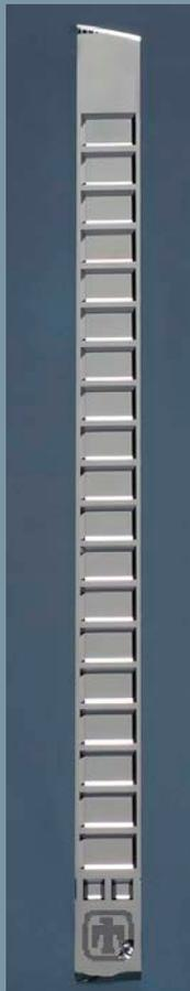
Figure 4: A Silicon Micromachined Dimensional Calibration Artifact "step gauge" diced from a wafer such as shown in (Figure 2). The wafer shown in Figure 2 can be diced to make 13 "step gauges."
