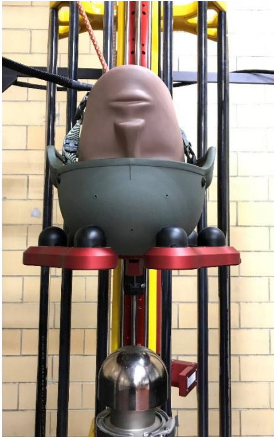
Figure 2-1. Mil-spec experimental setup, with hemispherical anvil.
