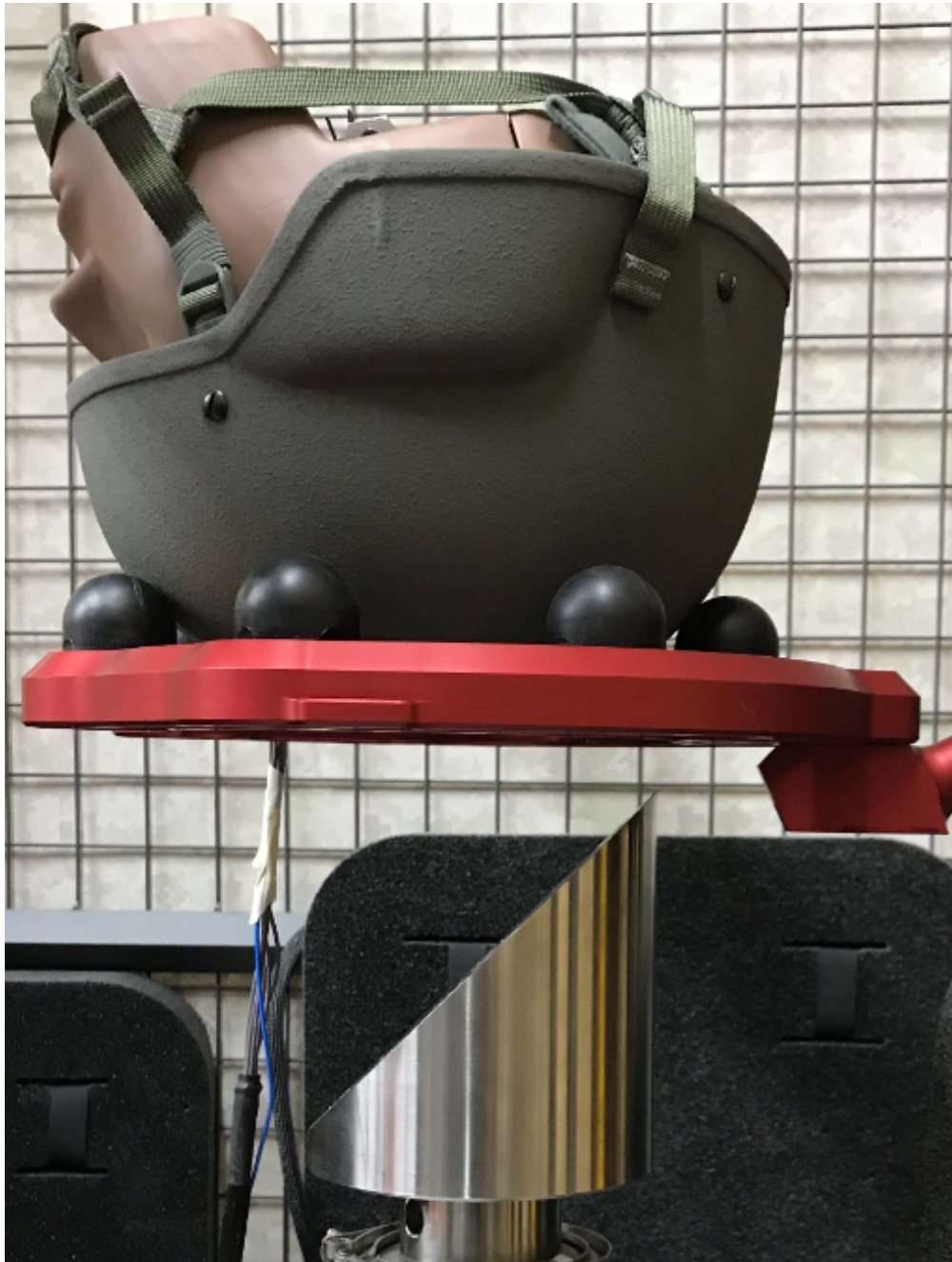
Figure 2-2. Modified mil-spec experimental setup, with flat, inclined anvil.
