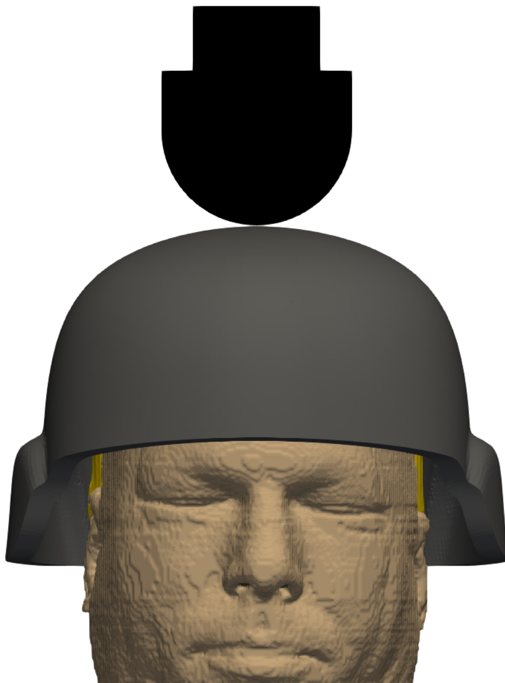
Figure 3-3. Frontal view of helmeted human model, impacting the hemispherical anvil.
