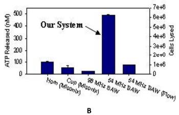
**Figure 2.** Acoustic lysing system. **A)** Actual Operating device with an attached microchannel **B)** Comparison of lysing systems as measured by ATP release. The ATP assay was linear from 102-108 cells/ml. The flow rate was 50  $\mu$ l/ml for rightmost case.
