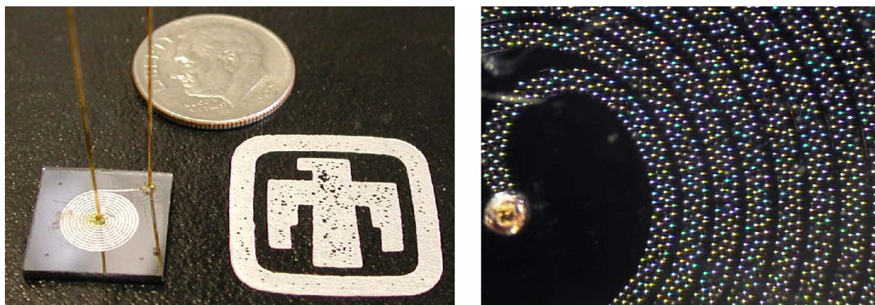
Figure 2. Left, micro-GC column filled with HayeSep D chromatography beads. Right, close up with Carboxen 1000 beads. Approximate column dimensions: 0.5" x 0.5" x 0.040" thick.
