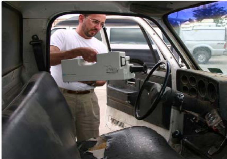
Figure 2. The MicroHound™ detects explosive with high and low vapor pressures.
