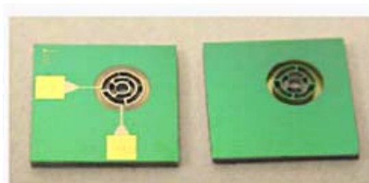
Figure 5. 3D-PC with flow perpendicular to the substrate surface. Front and rear sides of the die show an adsorbent support of cylindrical cylinders of Si, all suspended by a SiN membrane. The central part of the SiN membrane is etched open to allow flow through the device
