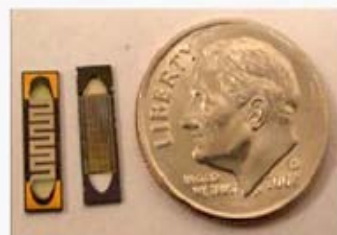
Figure 5. 3D-PC with flow perpendicular to the substrate surface. Front and rear sides of the die show an adsorbent support of cylindrical cylinders of Si, all suspended by a SiN membrane. The central part of the SiN membrane is etched open to allow flow through the device
