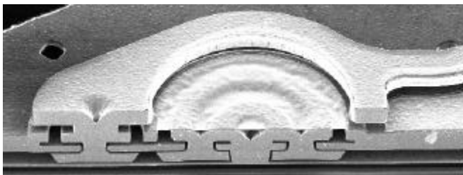
Figure 10. 2D Cross-section of a gear and pin joint
