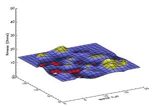
Figure 8. Source/drain contact resistance for 2  $\mu$ m x 2  $\mu$ m contacts to p-channel devices.
