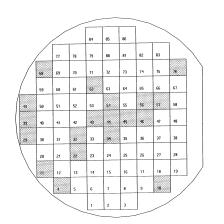
Figure 6. A wafer map from the first run showing functionality of wafer-level tests of combustible gas sensor devices. The unshaded devices are functional.
