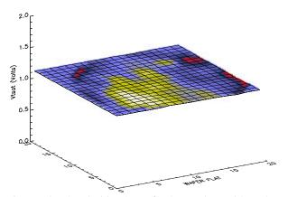
Figure 10. Threshold voltage for 2  $\mu$ m channel length, n-channel transistors.
