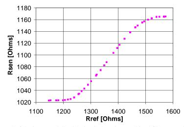
Figure 14. Under the control of the integrated CMOS circuit the micromachined filament resistance follows the reference resistance.
