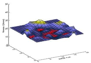
Figure 9. Metal to poly contact resistance.
