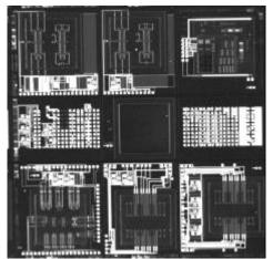
Figure 5. An photograph of the completed integrated MEMS/CMOS die illustrating the layout of the various sensors, resonators, test structures, and electronics.
