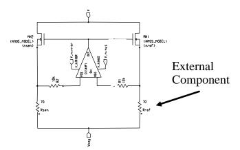
Figure 13. Schematic of the CMOS control circuit integrated with the micromachined sensing filament (labeled Rsen). For the purposes of testing, the micromachined reference resistance was replaced with a 10-turn potentiometer.
