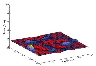
Figure 7. Source/drain contact resistance for 2  $\mu$ m x 2  $\mu$ m contacts to n-channel devices.
