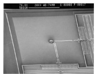
Figure 4. A three-level polysilicon structure (microengine) built in a trench. Here, the trench depth is approximately 12  $\mu$ m.
