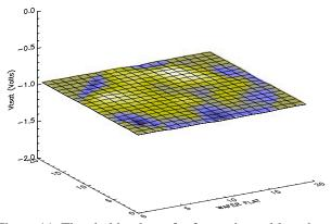
Figure 11. Threshold voltage for 2  $\mu$ m channel length, p-channel transistors.
