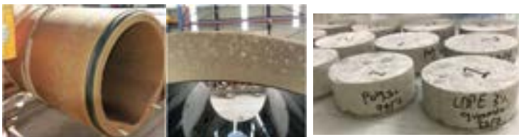
Meyer Polycrrete sewer pipes (left), JKT Group Polymer Concrete pipe, polymer modified concrete samples (Mohammed, 2022)
