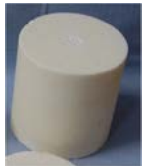
Figure ...: HITEC salt (Coastal Chemical) with 53% \text{KNO}_3 , 40% \text{NaNO}_2 , 7% \text{NaNO}_3 and a melting point 142°C (Minkley, 2018) – Not to be used in a rock salt underground repository environment due to chemical behavior.
