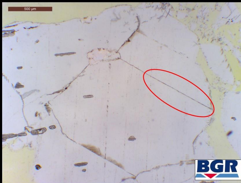
Microcracks in crushed salt raw material
