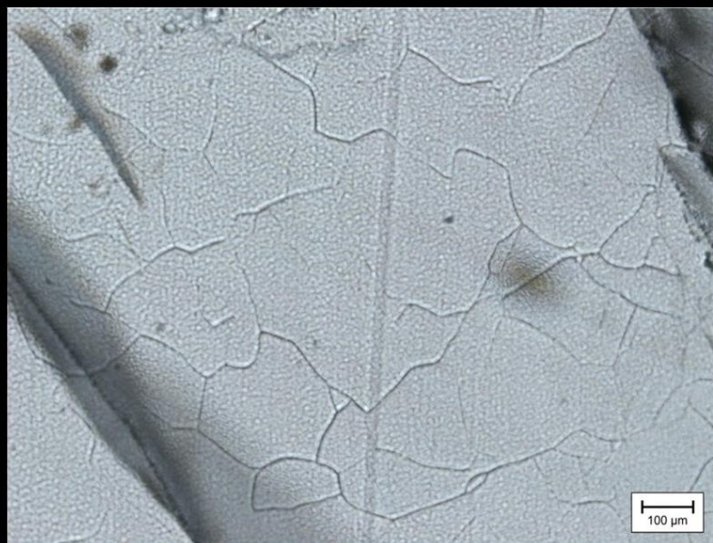
Subgrains in compacted crushed salt (oedometric compaction; 50°C, max. 30 MPa)
