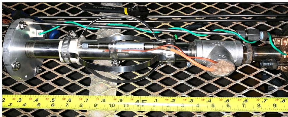
**Figure 17. Closeup of borehole closure gauge (heater on left, packer on right). Borehole closure produces a deflection of the springs attached to PEEK bushing (left side) which slides axially. The sliding is measured by an LVDT (connected by orange wire).**
