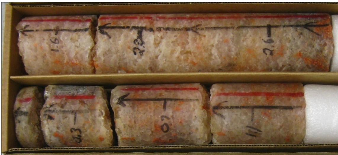
Figure 13. Photograph of 4-inch [10 cm] diameter core (H:SL, box 1), numbers written on core are feet measured from drift face.
