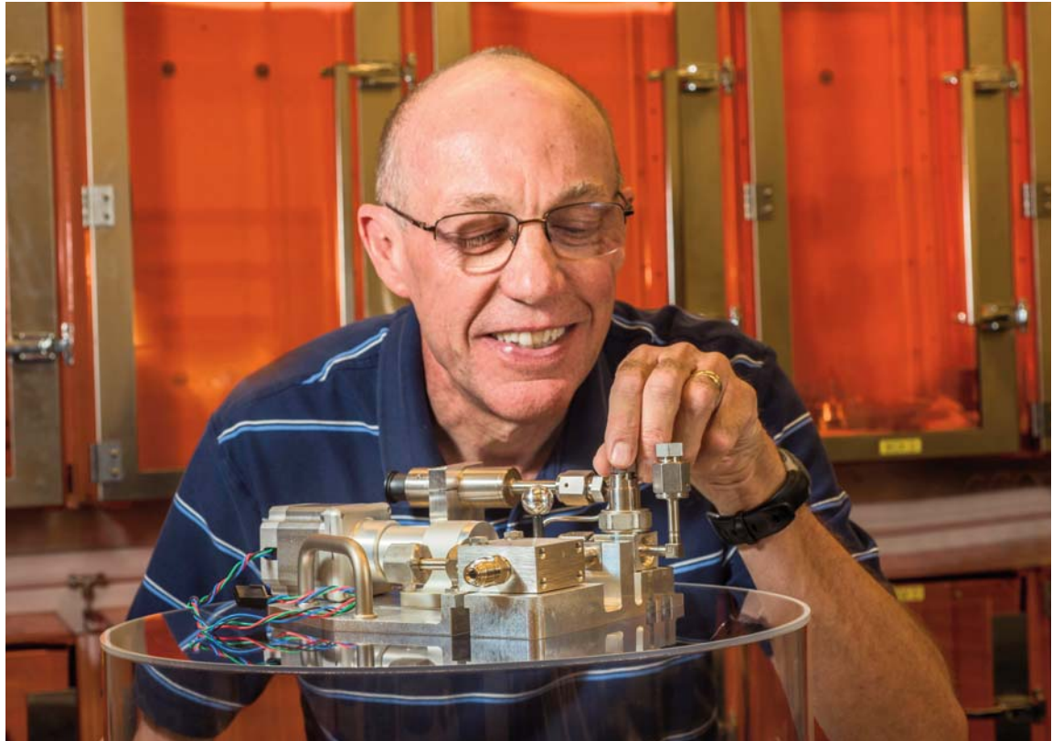
TRITIUM SHOT PI DEAN ROVANG checks out Z's tritium gas transfer system (Z-GTS), which was built in Sandia/California and filled with trace tritium (0.1 percent) at Sandia/New Mexico. (Photo by Randy Montoya)
