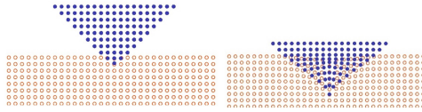
FIG. 4.1. Interpenetration in the case of an impactor striking the stationary target at 5 km/s.
