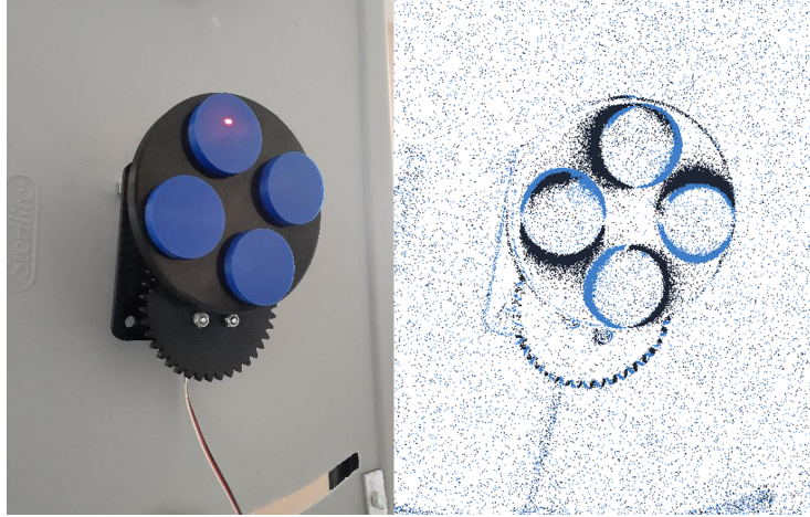
FIG. 1.2. Image comparison for frame-based image and binned event sensor capture using a Prophesee Gen 4. Blue represents positive pixel events where it got brighter and black represents negative events where the pixel darkened.
