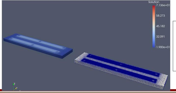
Left: Additive manufacturing simulation showing temperature in evolving geometry
