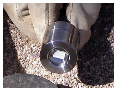
Figure 2. Weatherproof chemiresistor package that can be emplaced in a monitoring well or cone penetrometer.
