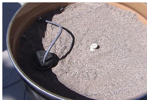
Figure 3. Top view of 55-gallon drum filled with sand. The contaminant reservoir is in the middle of the drum, and the sensor well is towards the outside.
