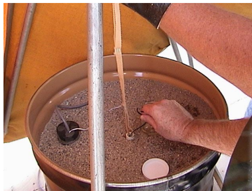
Figure 5. Emplacement of a TCE-soaked wick into the reservoir.
