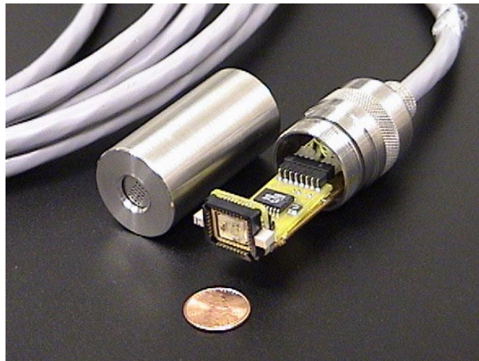
Figure 6. Integrated SAW probe for in-situ monitoring applications.
