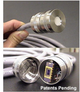
Weatherproof sensor package. The unique design and GORE-TEX ® membrane allows the enclosed chemiresistors to "sniff" chemicals in air, soil, and water environments.
