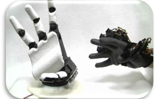
Robotic users have a need for a low-cost robotic hand that can perform highly dexterous tasks in a variety of hazardous environments. Sandia National Laboratories, in collaboration with Stanford University and Lunar, has developed The Sandia Hand for the DARPA-sponsored Autonomous Robotic Manipulation (ARM) Program to address this need. The Sandia Hand is low-cost, dexterous, and modular enabling it to support a variety of applications including:
