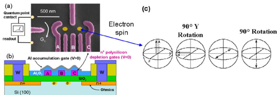
(a) scanning electron microscope image of Sandia's dual quantum dot structure fabricated in silicon (the dots suggest the approximate location of the electron position); (b) schematic cross section of the quantum dot structure showing the position of the single electron locations; and (c) schematic representation of spin manipulation using rotation and precession of two different spins.
