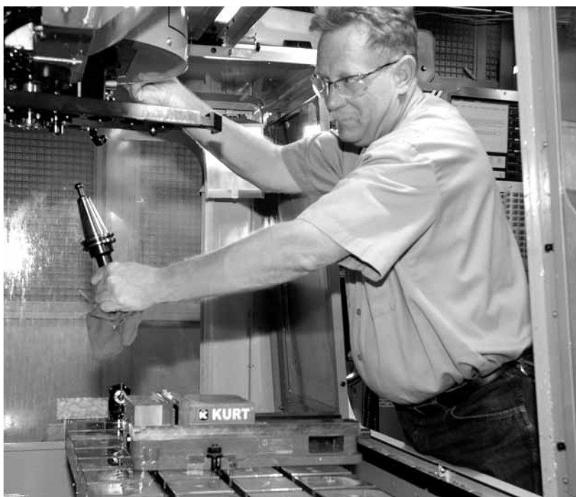
IT GOES IN THIS WAY — Tim Mitchell (2431) loads a cutting tool, this one intended for future use, into a new Haas milling machine's automatic tool changer. (Photo by Bill Doty)
