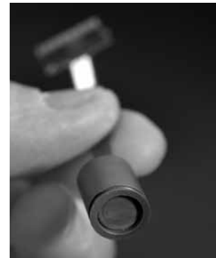
DETAIL of hydrogen sensor developed at Sandia and commercialized by H2scan.
