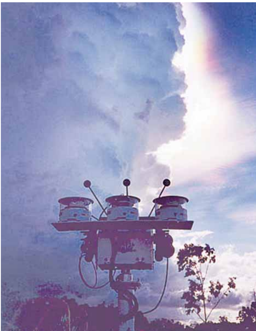
SKYWARD — A collection of radiometers at the Darwin, Australia, site continuously measures irradiance in cumulus clouds. Ground-based instruments will support the 2006 Tropical Warm Pool-International Cloud Experiment to describe the properties of tropical cirrus and the convection that leads to their formation.
