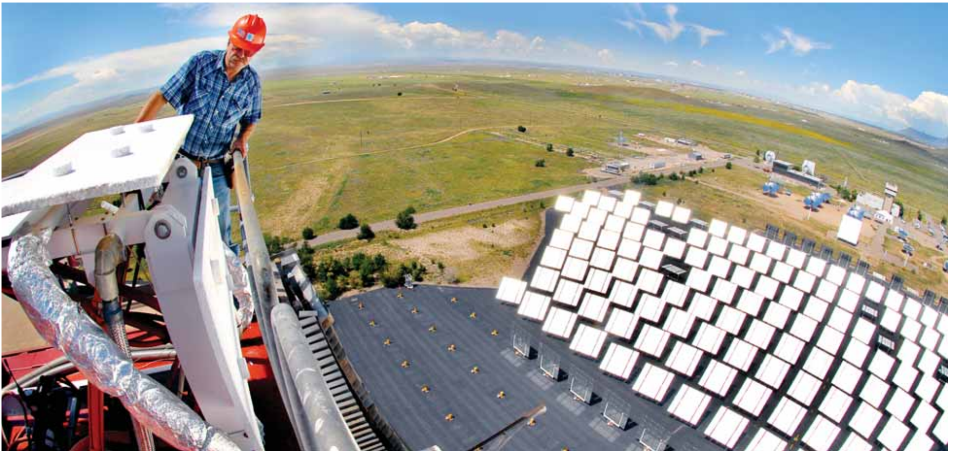
JOHN KELTON (6218) prepares samples for NASA's ablative shield materials test at the top of Sandia's solar tower. NASA chose the solar facility after determining it was the only
