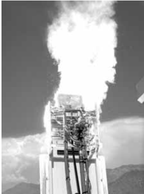
FLAME rises from material as it is superheated by the tightly focused beam produced by the solar tower's heliostat field. (Photo by Randy Montoya)
