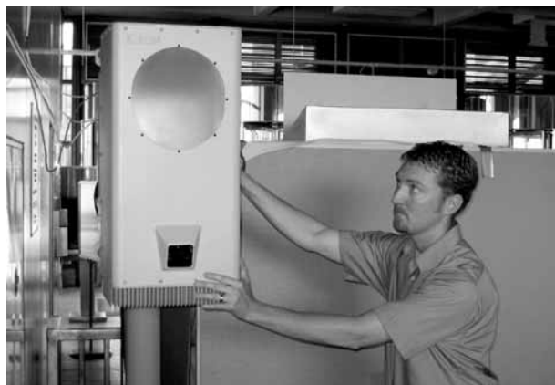
ERIC VARLEY (6418) sets up a passive millimeter-wave weapon detection system at the Port Authority of New York and New Jersey's Exchange Place Station.
