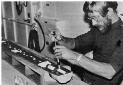
FROM THE OCEAN DEEP — A core sample taken from beneath 20,000 feet of North Pacific Ocean is examined as part of a program to determine feasibility of radioactive waste disposal in deep sea sediment.
