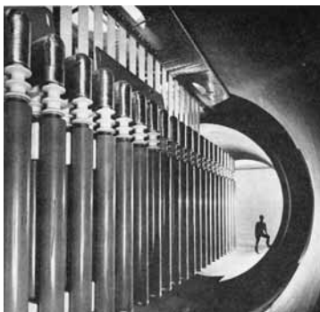
HERMES II capacitors will store a maximum of one million joules to provide the basic energy of the machine. The interior of the steel tank will be filled with 150,000 gallons of mineral oil.
