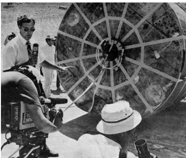
FIRST DROP TEST of the TRUPACT II waste container at Sandia's New Cable Site.
