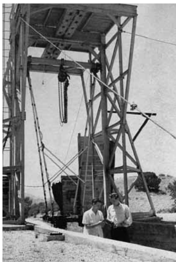
PENDULUM ENGINEERS—Standing before the rocket-powered pendulum in a Sandia technical area are Bill Duggin and Bob Hager. The device was used for shock testing.
