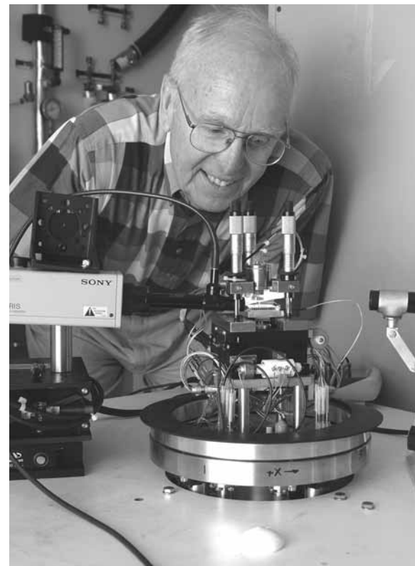
A NEW WAY OF SEEING — Jack Houston has used his own invention, the interfacial force microscope (recently enhanced with new capabilities) to study the effects of aging on complex polymer chains.
