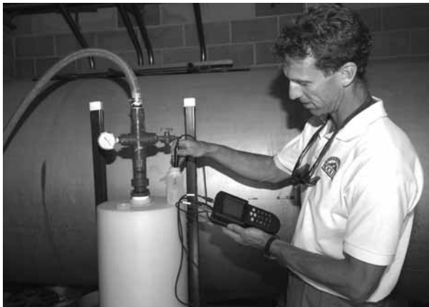
SANDIA RESEARCHER Brian Dwyer checks out arsenic removal equipment at Casa Angelica. The facility's well provides drinking and bathing water to 16 medically fragile children and young adults who live there.
