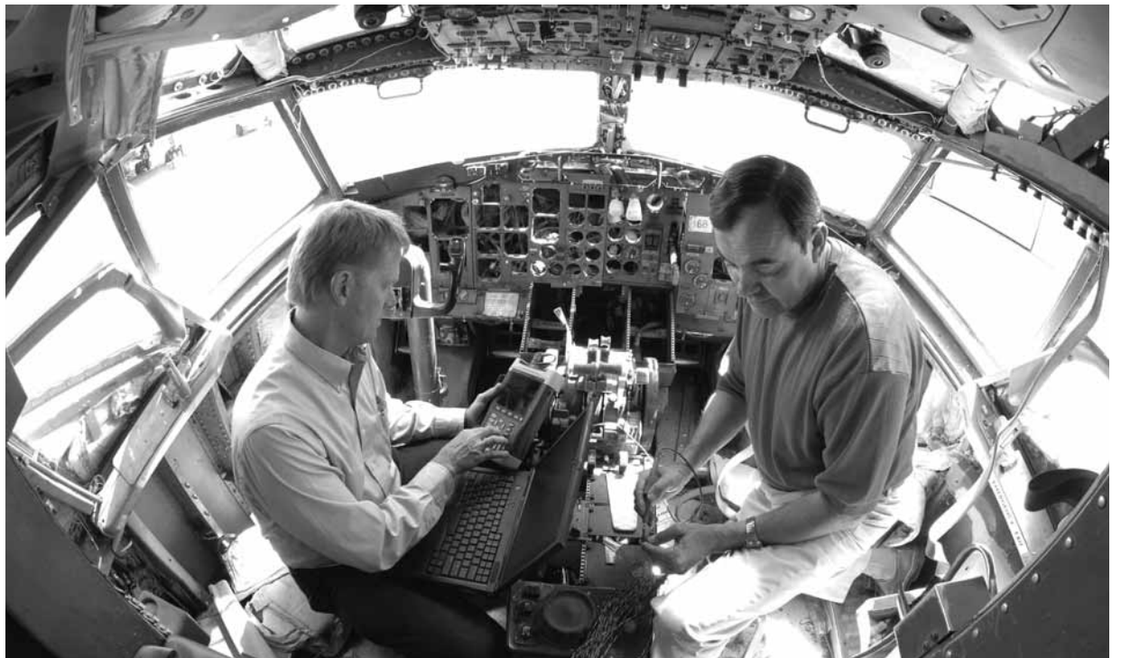
Mike Dinallo and Larry Schneider (left) prepare to employ the PASD diagnostic on a wiring bundle in the cockpit of a retired Boeing 737 at Sandia's FAA Airworthiness Assurance NDI Validation Center. (Photo by Randy Montoya)
