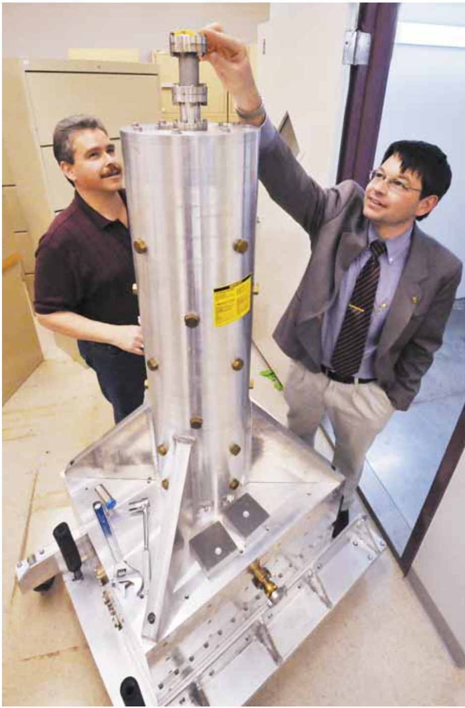
MERCURY ON THE MOVE — David Sanchez (2541) and Jay Hendricks from the National Institute of Standards and Technology examine a mercury manometer prior to its transport from Sandia to NIST in Gaithersburg, Md. (Photo by Randy Montoya)
