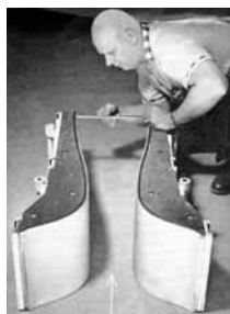
SUPERSONIC NOZZLE BLOCK being prepared for installation by Cecil Tolbert of the Experimental Aerodynamics Division.
