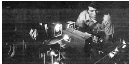
CARS FOR COMBUSTION — Coherent anti-Stokes Raman spectroscopy (CARS), demonstrated here by Larry Rahn of Applied Physics Division.
