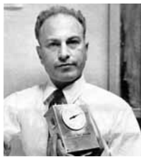
BLAST YIELD METER, held by its inventor Howard Sander, indicates yields of nuclear weapons detonated.
