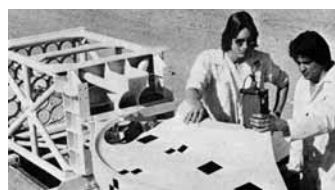
THE ELECTRICAL CONNECTIONS being checked on a segment of a turbine hub before the first sled test.
