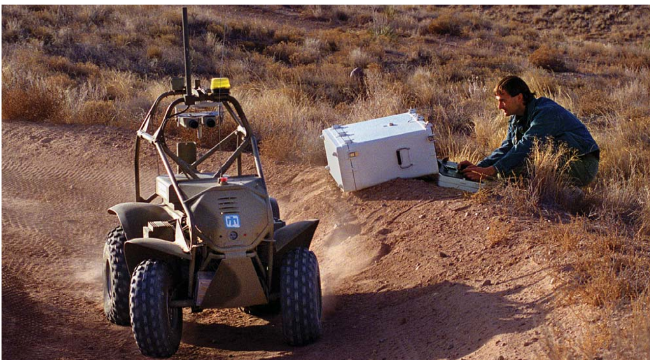
DIXIE BATTLEFIELD SCOUT ROBOT is able to navigate through a variety of terrain, including snow and ice. Former Sandian Bryan Pletta is at the controls. (Photo by Randy Montoya)
