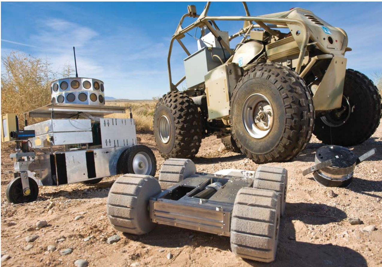
SANDIA INTERIOR ROBOT, or SIR, (left) was developed in 1985 and was one of the first truly autonomous interior robots; Dixie (upper right) was created in 1987 as one of the earliest battlefield scout robots; and Hopping Robots (lower right) are able to navigate autonomously onto or over obstacles. (Photo by Randy Montoya)
