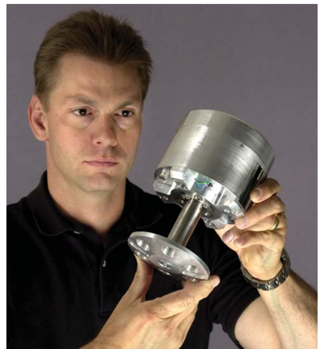
GARY FISCHER holds one of the combustion-powered hopping robots developed at Sandia. (Photo by Randy Montoya)
