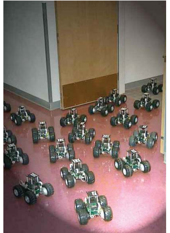
SANDIA NETBOTS were, at the time, the largest team of cooperating small robots ever developed. (Photo by Randy Montoya)
