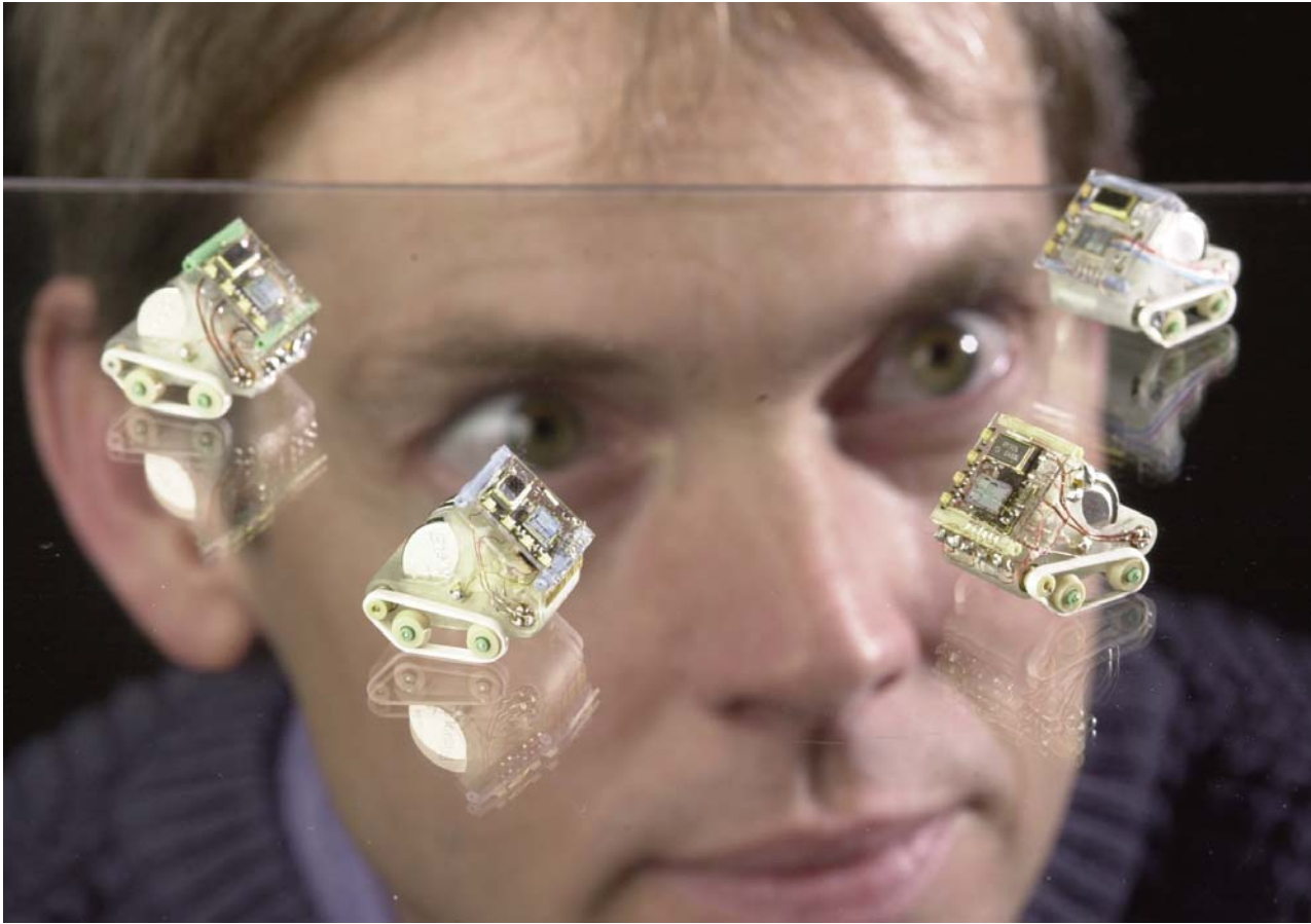
SANDIAN DOUG ADKINS examines superminiature robots, which are ¼ cubic inch and weigh less than an ounce, debuted in 2001. At the time, they were possibly the world's smallest autonomous untethered robots ever created. (Photo by Randy Montoya)
