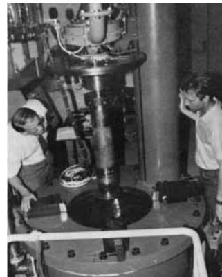
EXAMINING THE W82 test unit suspended on the shaft from the turbine above the six-foot-deep containment tank are Pat Gildea (left) and Guy Prescott. These test units are spun up to 18,000 rpm on the spin-test device.
