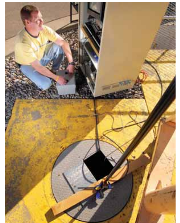
A DEFT TOUCH — Don Hanson (1382) controls the movements of Swarmy the robot in an old wastewater storage tank 26 feet underground, an environment not safe for human entry. (Photo by Randy Montoya)
