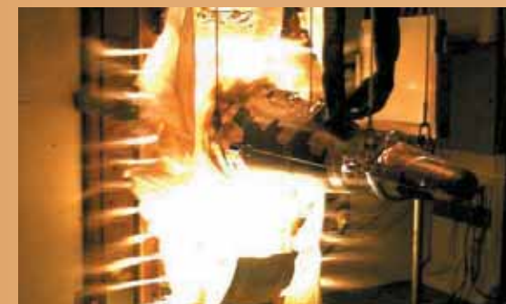
A SERIES OF ULTRABRIGHT LIGHT SOURCES ignites the sprayed-on explosive coating on a W76 test article during a test at the Light Initiated High Explosive facility.
