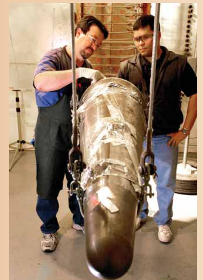
GARY RIVERA (left photo) prepares chemicals used in spray-on explosive coating at the LIHE facility. In photo at right, Dan Dow and Gary (both 2554) prepare a test article for an LIHE test.
