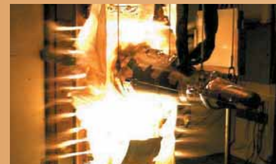
A SERIES OF ULTRABRIGHT LIGHT SOURCES ignites the sprayed-on explosive coating on a W76 test article during a test at the Light Initiated High Explosive facility.
