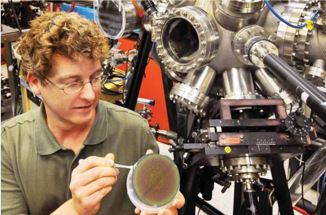
INTERSTELLAR FILMS — Tom Friedmann (1112) checks out a sample diamond-like carbon film he created for the low-energy sensor (IBEX-Lo) on board NASA's Interstellar Boundary Explorer (IBEX). Thirty films are on board the IBEX. (Photo by Randy Montoya)
