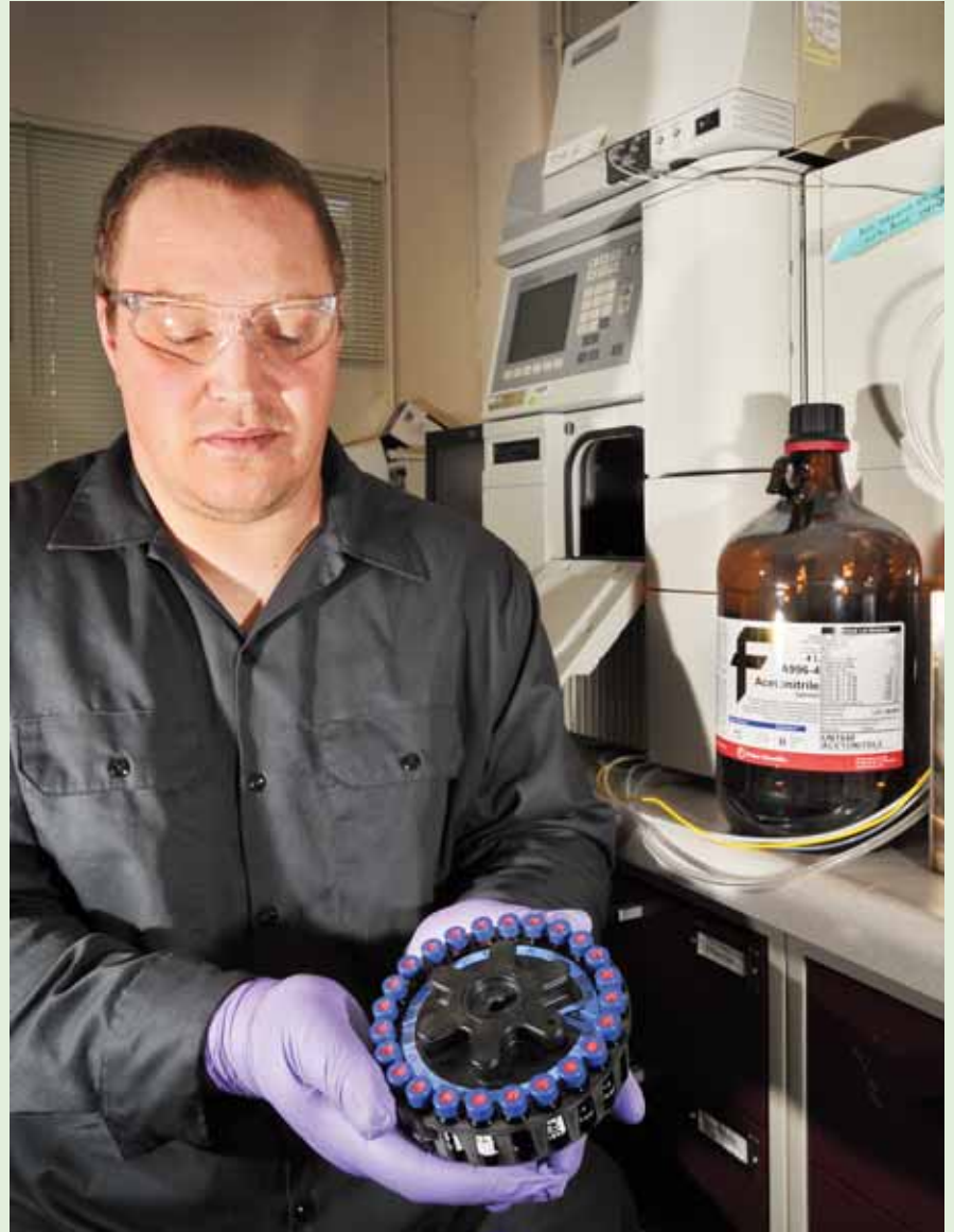
STEVE CHRISMAN displays a rack of chemicals prepared for separation in the high-performance liquid chromatography device (in the background). Steve routinely uses acetonitrile in the laboratory as a key tool in the chemical separation process. The global shortage of acetonitrile has researchers scrambling for alternatives. (Photo by Randy Montoya)
