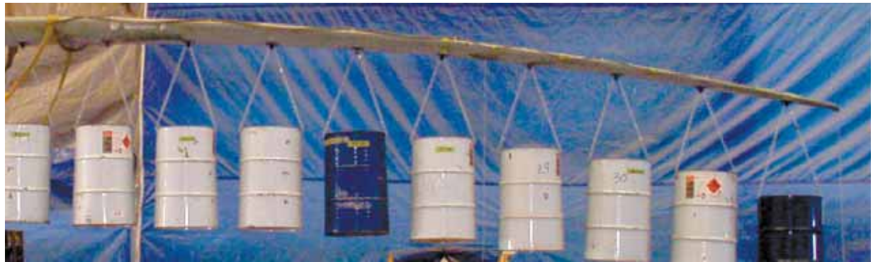
PROOF LOAD TESTING on new Sweep Twist Adaptive Rotor blade using 55-gallon-drums to test blade strength.
