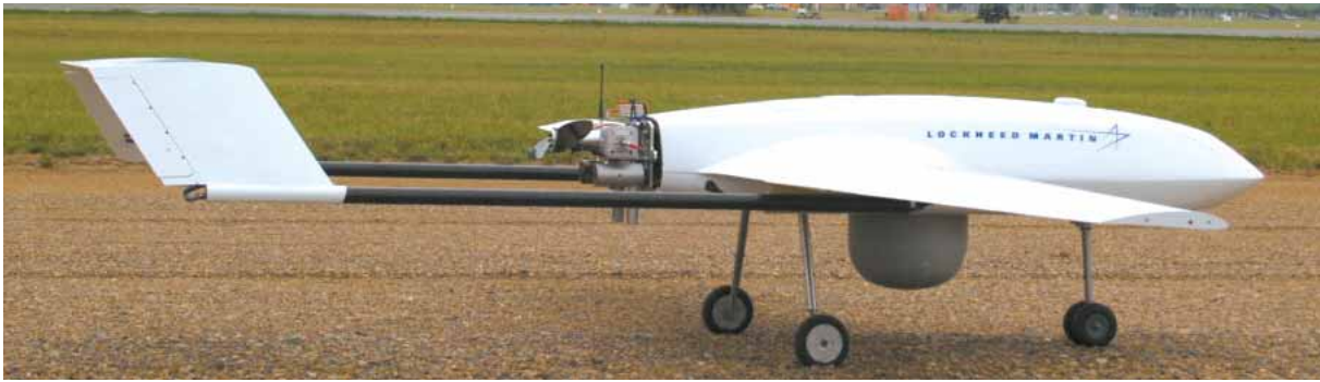
MINISAR SYSTEM developed at Sandia undergoes flight-testing on a Lockheed Martin SkySpirit unmanned aerial system during tests last fall in Minnesota. (Photo courtesy of Lockheed Martin)
