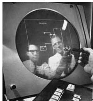
A LIGHT PEN was used to sketch an electrical diagram on the Sandia computer graphics system.
