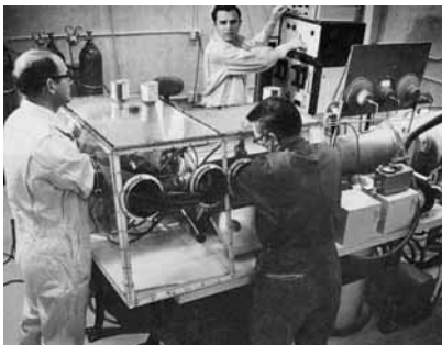
PREPARING TO BLAST A MICROSPHERE of plutonium dioxide in the plasma jet facility in Bldg. 849.
