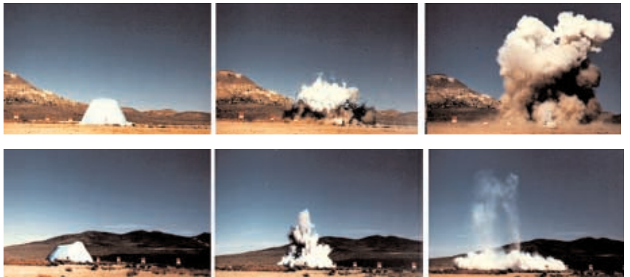
BLAST TESTS without foam mitigation (top row) and with foam mitigation (bottom row) show differing dispersals.
