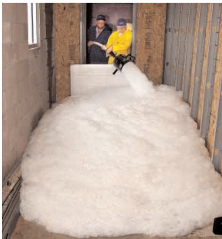
BLAST FOAM — Weldon Teague, left, and John Fulton (both 5817) fill up a room with a blast-mitigation and chem-bio-rad-containment foam a Sandia team wants to put into the hands of first-responders. (Photo by Randy Montoya)
