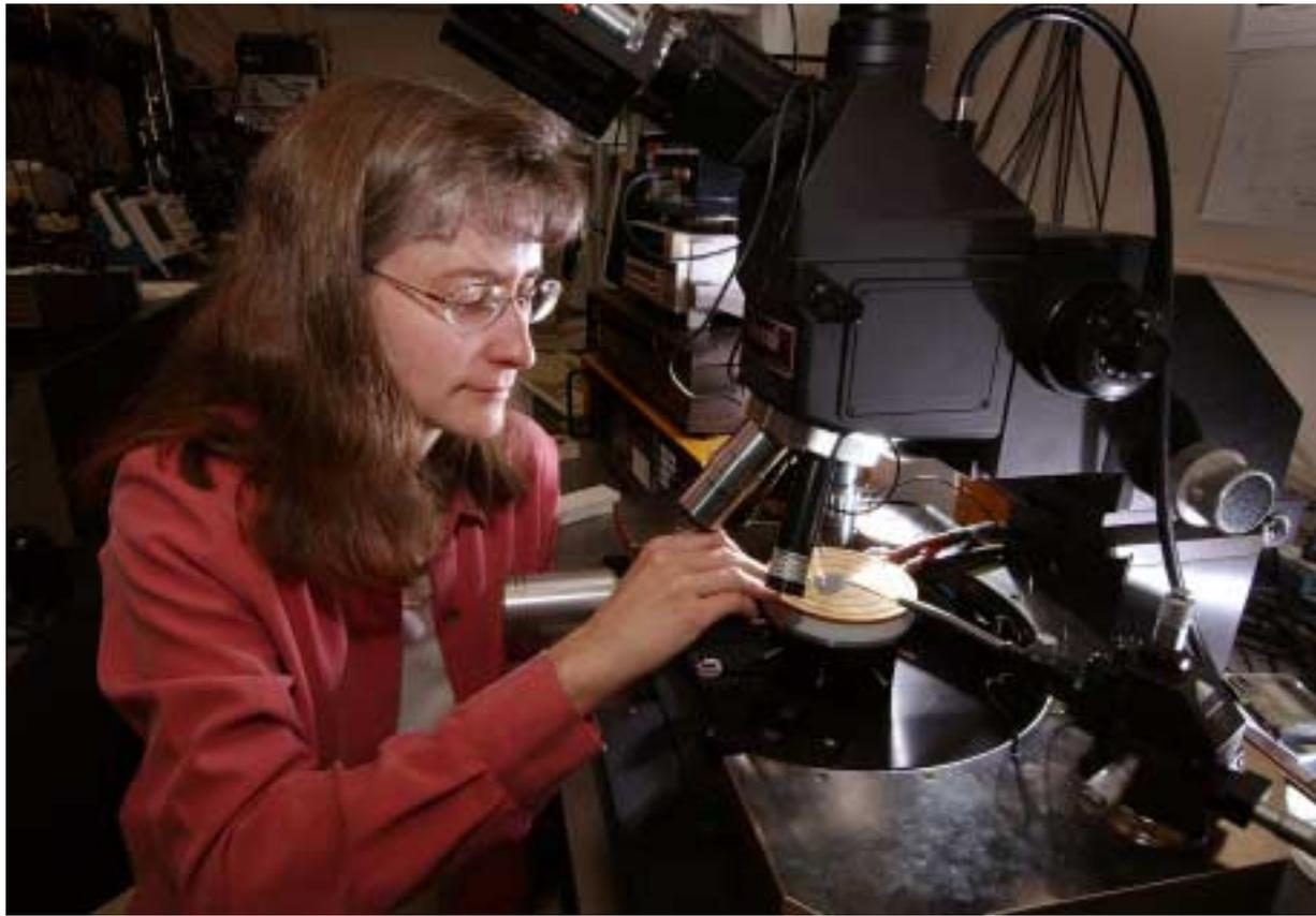
NEW UV LEDs — Sandia researcher Mary Crawford tests the output of an ultraviolet light-emitting diode developed by a Labs team that set new records. (Photo by Randy Montoya)
