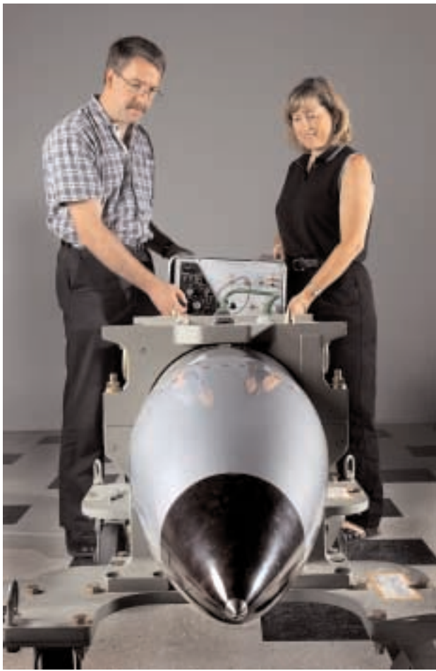
ELECTRONICS EXAM — David Clements and Beth Connors test a B61-4 Type 3E trainer using an F-111 Aircraft Monitor and Control (AMAC) package that simulates the electronic control system of several types of US military aircraft. (Photo by Randy Montoya)
