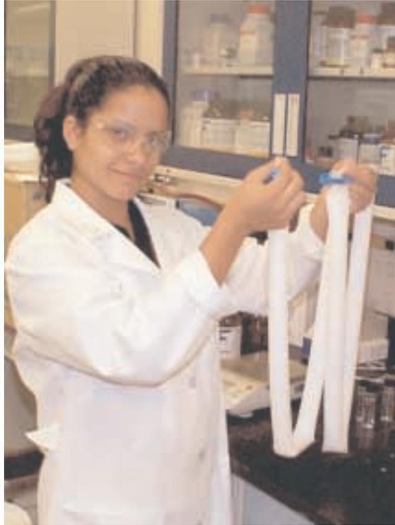
STUDENT MARLENE AXNESS holds a dialysis tube or "haggis" filled with hydrotalcite. After dialysis, filtration, and firing, the hydrotalcite is loaded into columns where it removes anions such as chloride, carbonate, and sulfate from brackish water.
