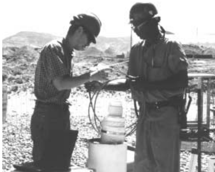
FIELD TEST — Cliff Ho (6115, left) and Henry Bryant (6134) deploy a chemiresistor package at the Sandia Chemical Waste Landfill as part of a field test.
