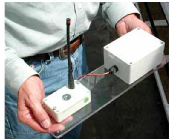
FORTY-TWO SENSOR DEVICES such as this will provide a stream of data to researchers on temperature, humidity, light intensity, and barometric pressure at multiple sites throughout the greenhouse.
